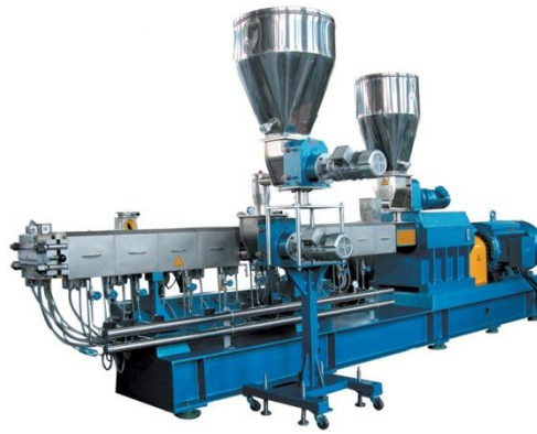
(2) Hot Melt Extrusion Equipment
