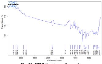
Fig. 11: FTIR Spectrum of pure drug.
