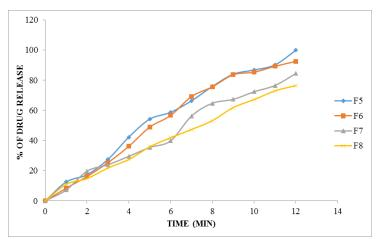
Fig. 5: Dissolution data of bupropion Floating tablets containing xanthan gum.
