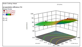
Fig. 6: Response surface plots for the effect of amount of stearic acid and PEG 4000 on % entrapment efficiency.
