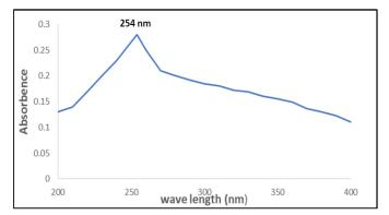
Fig. No. 1: Uv Spectrum of nifedipine in phosphate buffer (pH 7.4).
