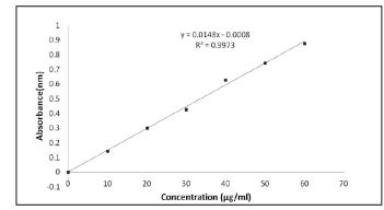
Fig. No. 2: Standard calibration curve of nifedipine in pH 7.4 Phosphate Buffer.
