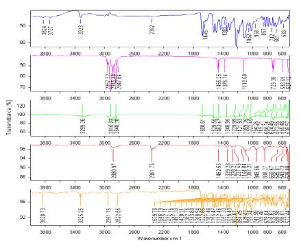
Fig. no. 3: FTIR spectrum of Nifedipine, Paraffin wax, Stearic acid, PEG 4000, and physical mixture (Nifedipine + Paraffin wax + Stearic acid + PEG 4000).
