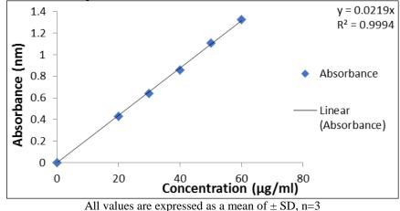
Fig 3: Standard calibration curve of Melampodium extract in phosphate buffer pH6.8 at 220nm.
