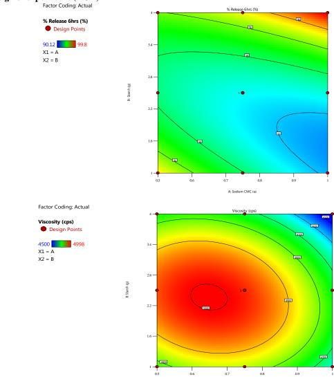
Fig. 5: counter plot showing the effect of sodium CMC and starch on (a)percentage release and (b) viscosity.
