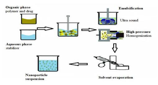
Fig. 2: Nanoparticle preparation using emulsion solvent evaporation methods.
