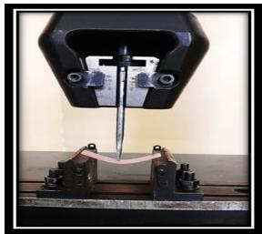
Figure 3: Flexural strength test using Universal testing machine.
