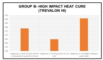
Figure 6: Mean flexural strength of high impact heat cure denture base resin after employing the three different cooling procedures.
