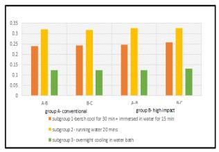
Figure 4: dimensional changes of group A- conventional and group B- high impact the high impact heat cure resin (TREVALON HI) after employing the cooling procedures.
