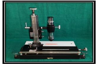
Figure 2: Measurement of linear dimensional change using travelling microscope.
