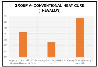
Figure 5: Mean flexural strength of conventional heat cure denture base resin after employing the three different cooling procedures.
