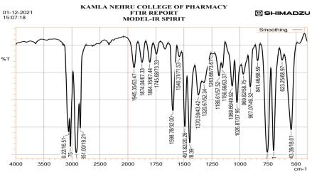
Figure 3: FTIR Spectrum of Naratriptan HCl.
