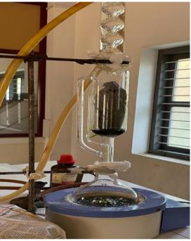
Fig. No. 3: Soxhlet extraction.
