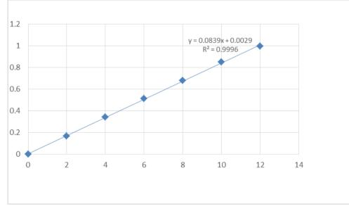
Fig.3: Calibration curve for Ciprofloxacin Hydrochloride at 272 nm by Zero order Spectroscopy.
