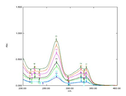
Fig. 3: Zero order overlain spectra of Ciprofloxacin Hydrochloride at 272 nm.
