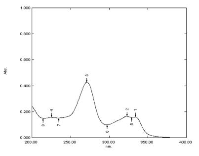
Fig. 2: Zero order spectra of Ciprofloxacin Hydrochloride showing absorbance at 272 nm.
