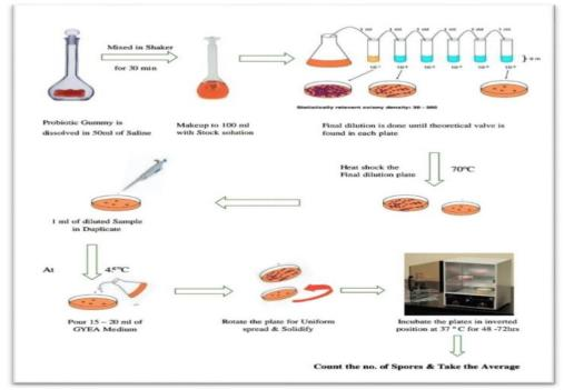
Fig.3: Schematic Representation of TVSC Plate for Probioticgummies.
