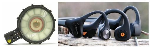
Figure-17: Planar magnetic driver and Magnetostriction headphones.
