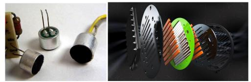
Figure-16: Electret and planar magnetic microphone.
