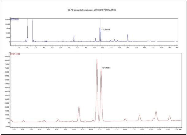
Figure 3: GC-FID chromatogram of detected 1,8-cineole in NEWCHARM<sup>®</sup> GEL (R<sub>t</sub> 10.79).
