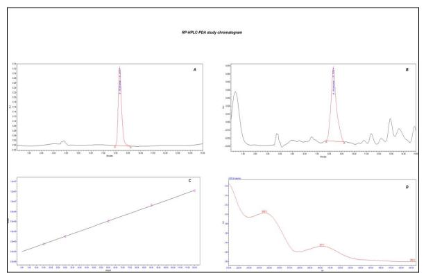
Figure 4: RP-HPLC-PDA-chromatograms (245 nm). (A) Standard chromatogram of  $\beta$ -asarone (R<sub>t</sub> 8.30). (B) Chromatogram of detected  $\beta$ -asarone in NEWCHARM<sup>®</sup> GEL sample (R<sub>t</sub> 8.30). (C) Linearity curve for the developed method of  $\beta$ -asarone. (D) UV spectrum of  $\beta$ -asarone in standard and samples of NEWCHARM<sup>®</sup> GEL.
