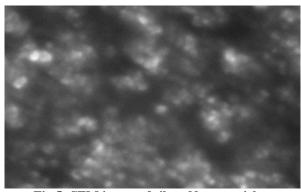
Fig.5: SEM image of silver Nanoparticles.
