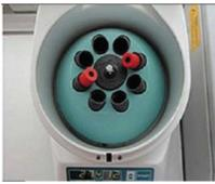
Figure 3: A specific centrifuge with a motor turning at alternated and controlled speed from 2,400 to 2,700 rpm for 12 minutes.
