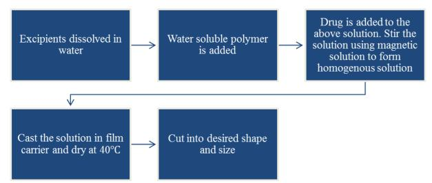
Figure 1: Flowchart for the process of solvent casting method.
