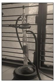
Fig. 2: Soxhlet extraction.
