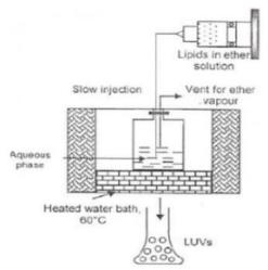
Fig. No. 09: Preparation of liposomes by Ether injection method.
