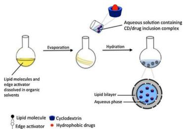
Fig. No. 08: Schematic representation of preparation of liposomes by thin film hydration technique/ Hand shaken MLV'S.
