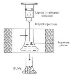
Fig. No. 10: Preparation of liposomes by Ethanol injection method.<sup>[29,28]</sup>
