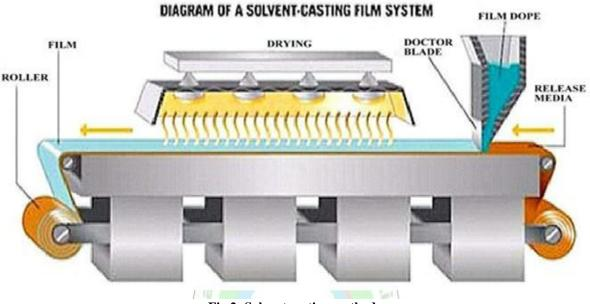
Fig 2: Solvent casting method.
