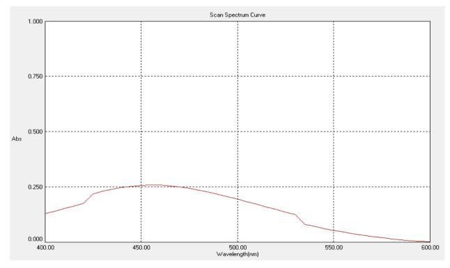
Figure [2]: Absorption Spectra of 12 3µg /ml of Triprolidine Hydrochloride.
