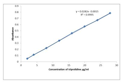
Figure [3]: Calibration Graph of Triprolidine Hydrochloride.
