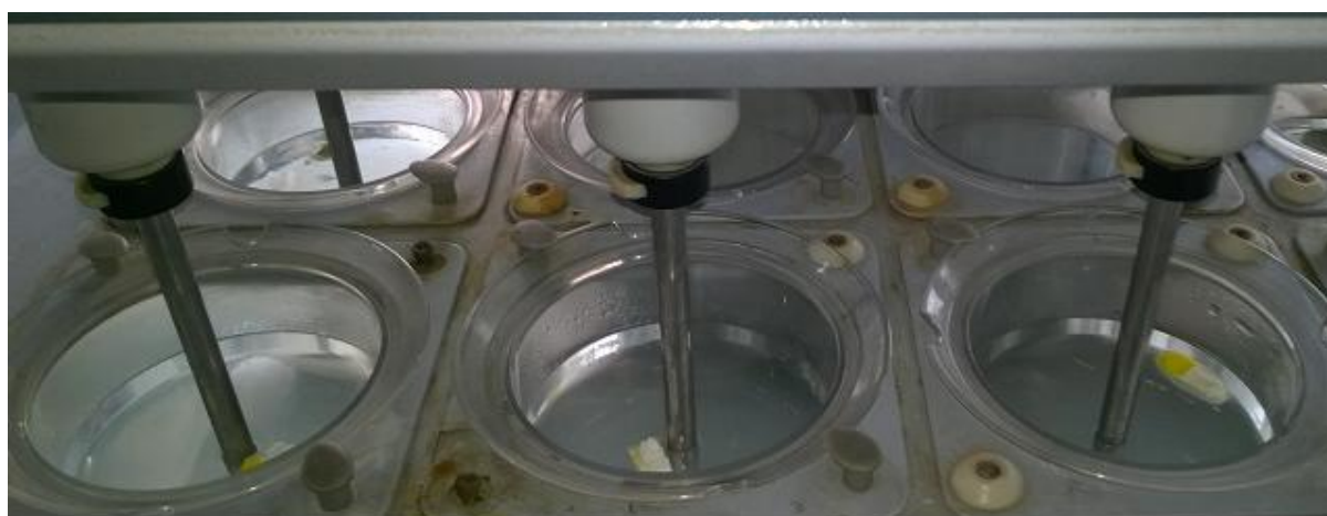
Figure 4: F1, F2, F3 remained buoyant in first hour.
