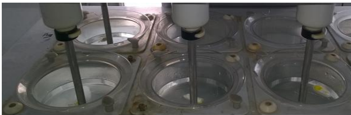
Figure 7: F1, F2, F3 remained buoyant in fourth hour. Gel formed by F1 starts to loosen its strength whereas F2 has firmed gel. F3 has formed firmed gel.
