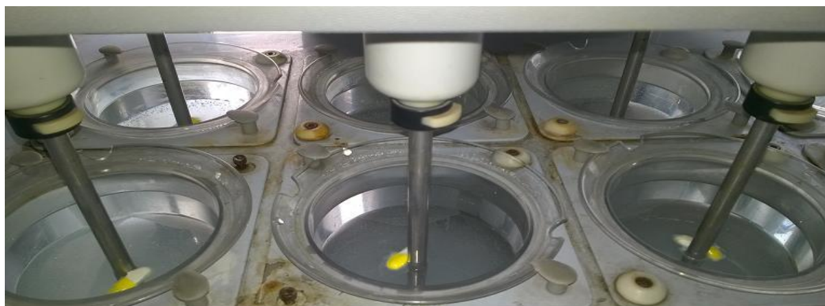
Figure 4: F1, F2, F3 remained buoyant in first hour.
