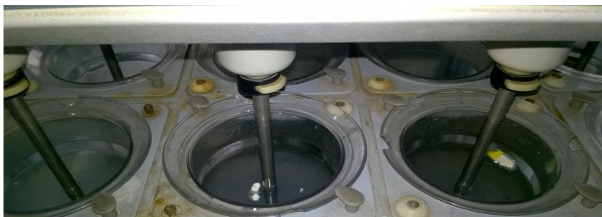
Figure 8: F2, F3 remained buoyant in fifth hour. Gel formed by F1 disappeared whereas gelled formed by F2 and F3 is firmed.
