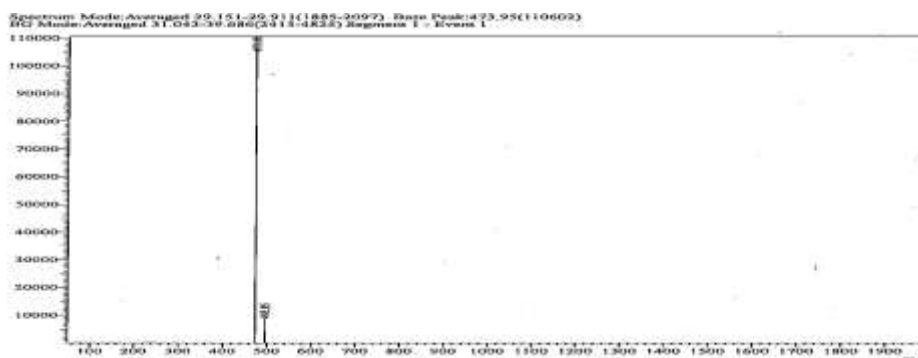
Fig-2 Mass spectral behavior of peak due to unspecified impurity at RRT 1.23.
