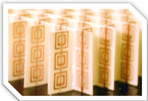
Figure 6 – "Photograph of [a] left-handed metamaterial (LHM) sample. The LHM sample consists of square copper split ring resonators and copper wire strips on [fibre] glass circuit board material. The rings and wires are on opposite sides of the boards, and the boards have been cut and assembled into an interlocking lattice." xiv
