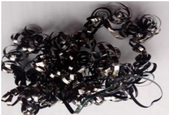
(e) At v_c = 315 m/min, s_0 = 0.08 m/min, & t = 2.05 mm
