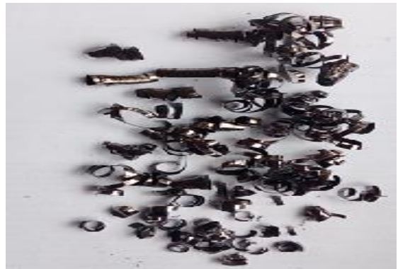
(f) At v_c = 315 m/min, s_0 = 0.1 m/min, & t = 2.05 mm
