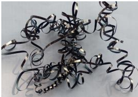
(i) At v_c = 240 m/min, s_0 = 0.08 m/min, & t = 2.05 mm
