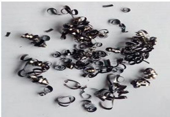
(i) At v_c = 240 m/min, s_0 = 0.08 m/min, & t = 2.05 mm
