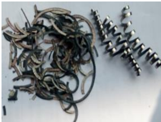
(k) At v_c = 240 m/min, s_0 = 0.12 m/min, & t = 2.05 mm
