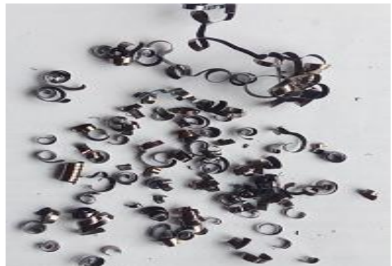
(j) At v_c = 240 m/min, s_0 = 0.1 m/min, & t = 2.05 mm
