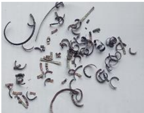
(a) At v_c = 410 \text{ m/min} , s_o = 0.08 \text{ m/min} , & t = 2.05 \text{ mm}
