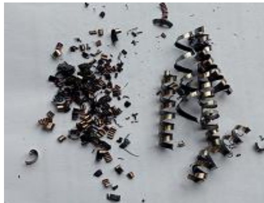
(l) At v_c = 240 m/min, s_0 = 0.14 m/min, & t = 2.05 mm
