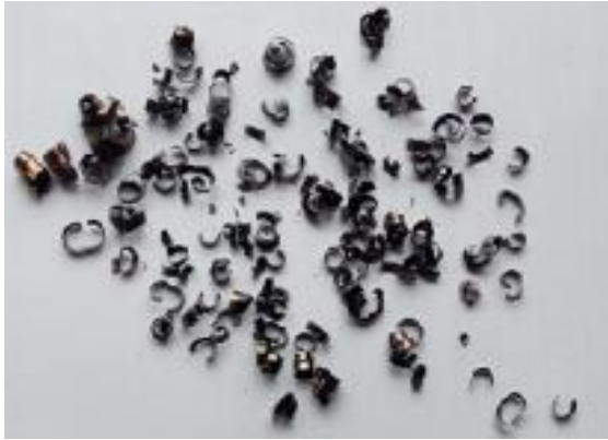
(c) At v_c = 410 m/min, s_0 = 0.12 m/min, & t = 2.05 mm
