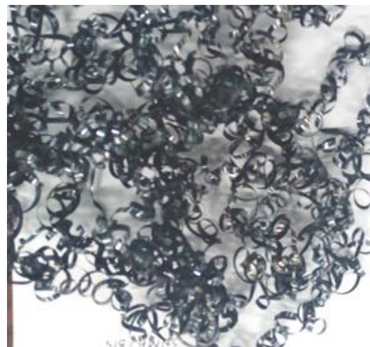
(f) At v_c = 315 m/min, s_0 = 0.1 m/min, & t = 2.05 mm
