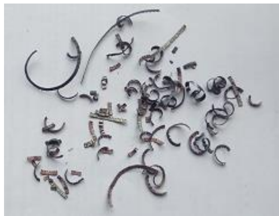
(b) At v_c = 410 \text{ m/min} , s_o = 0.1 \text{ m/min} , & t = 2.05 \text{ mm}
