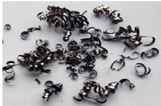
At v_c = 315 m/min, s_0 = 0.1 m/min, & t = 2.05 mm
