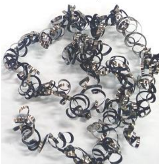
(c) At v_c = 410 m/min, s_0 = 0.12 m/min, & t = 2.05 mm
