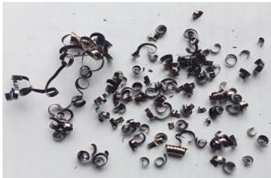
At v_c = 315 m/min, s_0 = 0.08 m/min, & t = 2.05 mm
