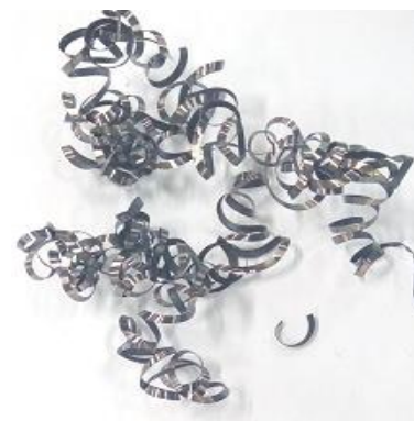
(l) At v_c = 240 m/min, s_0 = 0.14 m/min, & t = 2.05 mm
