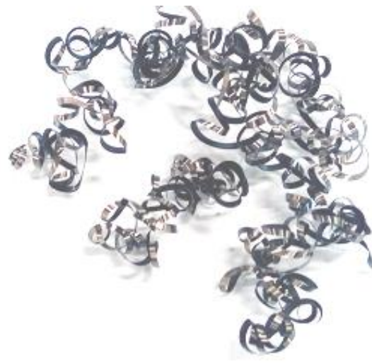
(h) At v_c = 315 m/min, s_0 = 0.14 m/min, & t = 2.05 mm
