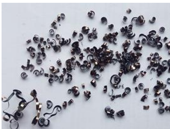
(c) At v_c = 410 \text{ m/min} , s_o = 0.12 \text{ m/min} , & t = 2.05 \text{ mm}
