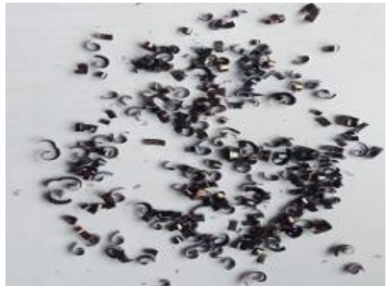
(h) At v_c = 315 m/min, s_0 = 0.14 m/min, & t = 2.05 mm
