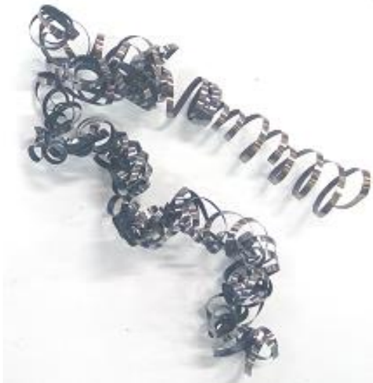
(a) At v_c = 410 m/min, s_0 = 0.08 m/min, & t = 2.05 mm
