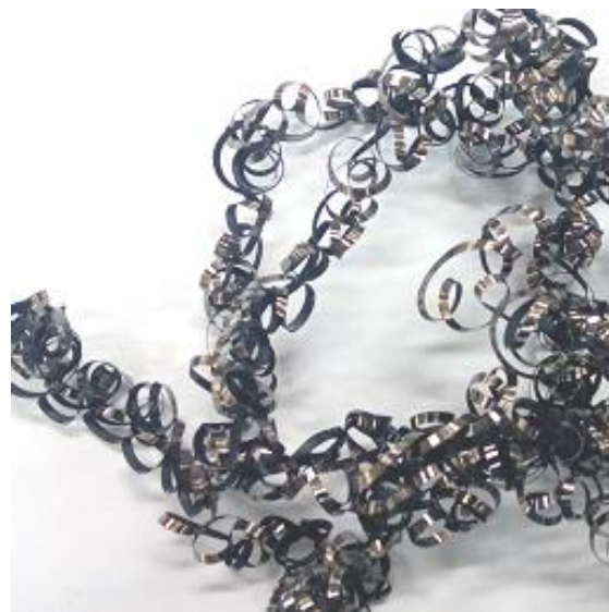
(b) At v_c = 410 m/min, s_0 = 0.1 m/min, & t = 2.05 mm
