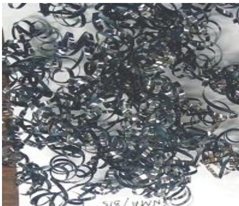
(i) At v_c = 240 m/min, s_0 = 0.08 m/min, & t = 2.05 mm
