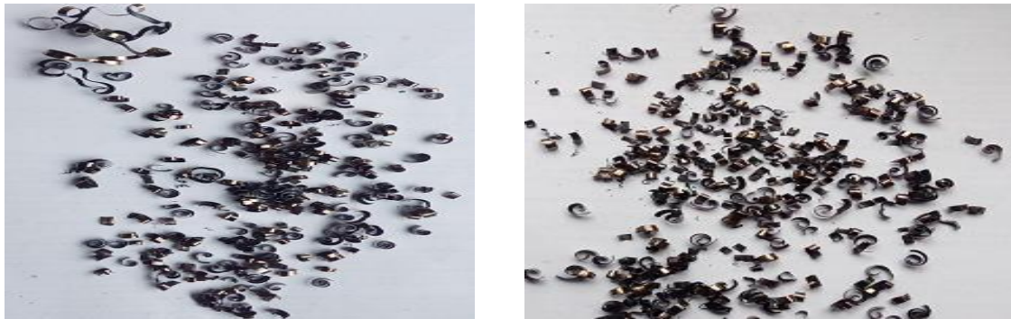
(k) At v_c = 240 m/min, s_0 = 0.12 m/min, & t = 2.05 mm (l) At v_c = 240 m/min, s_0 = 0.14 m/min, & t = 2.05 mm
