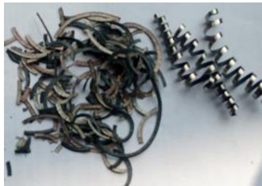
(j) At v_c = 240 m/min, s_0 = 0.1 m/min, & t = 2.05 mm
