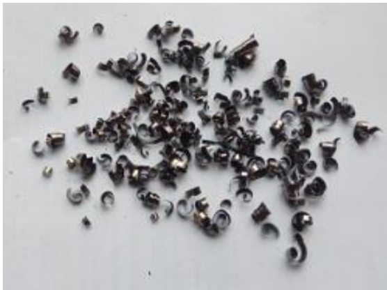
(g) At v_c = 315 m/min, s_0 = 0.12 m/min, & t = 2.05 mm
