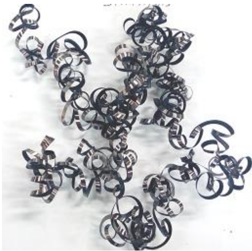
(g) At v_c = 315 m/min, s_0 = 0.12 m/min, & t = 2.05 mm
