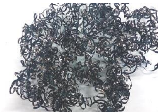
(k) At v_c = 240 m/min, s_0 = 0.12 m/min, & t = 2.05 mm
