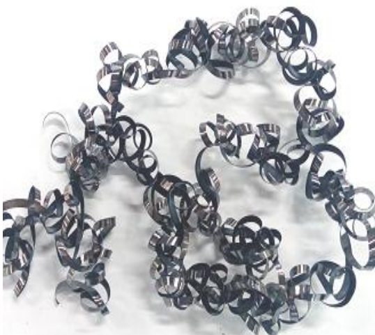
(e) At v_c = 315 m/min, s_0 = 0.08 m/min, & t = 2.05 mm
