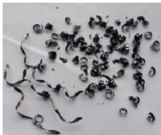
(b) At v_c = 410 \text{ m/min} , s_0 = 0.1 \text{ m/min} , & t = 2.05 \text{ mm}
