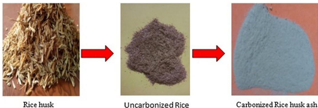
Figure 2. Secondary reinforcement: rice husk ash.
