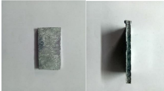
Figure 2. After fabrication, top and side view of metal matrix composite (MMC).
