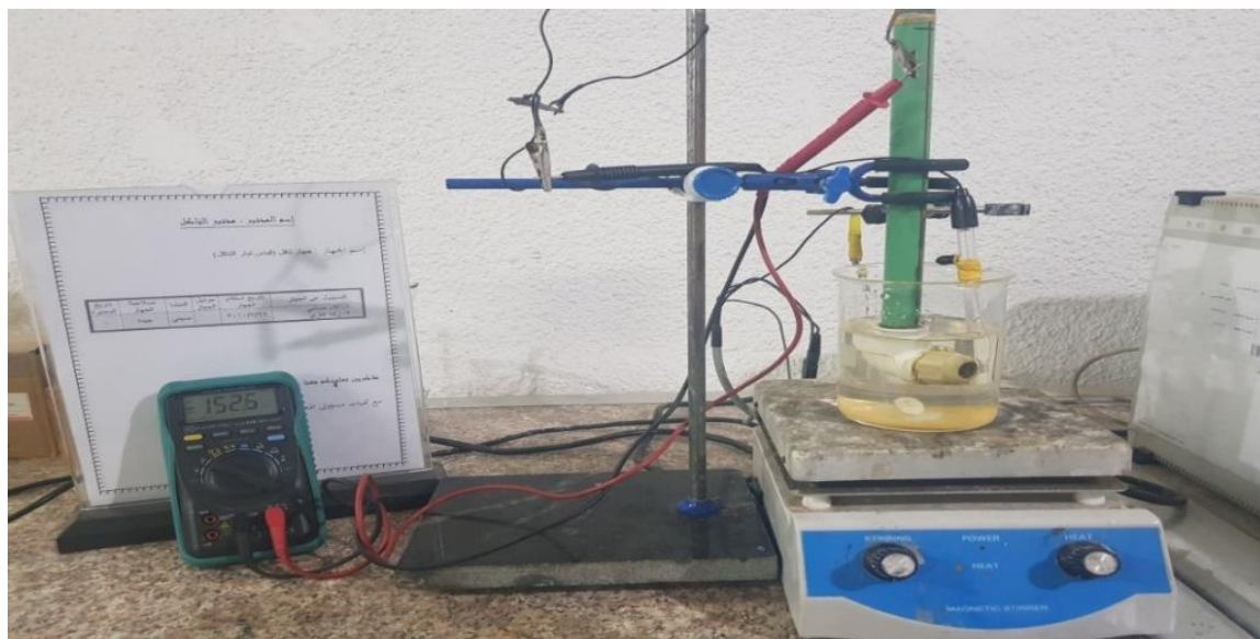
Figure 5. Schematic setup for measurement of open circuit potential.
