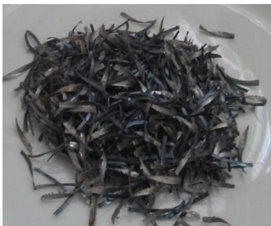
Figure 5. (a) Pozzolanic materials curves for particle size distribution, (b) Jagged Steel Chips [16, 18].
