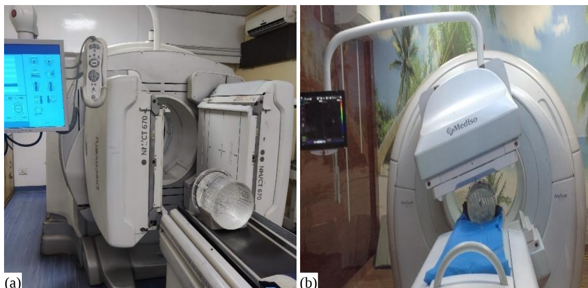
Figure 2. The experimental configuration of the Jaszczak phantom in GE and MEDISO SPECT/CT (a) Dual-headed GE SPECT/CT and (b) dual-headed MEDISO SPECT/CT.
