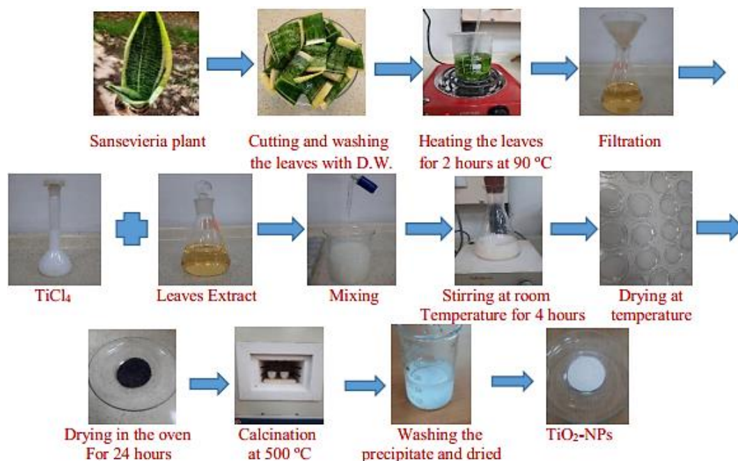
Figure 1. Steps of preparation of titanium dioxide nanoparticles (TiO 2 -NPs) using Sansevieria plant (SP).
