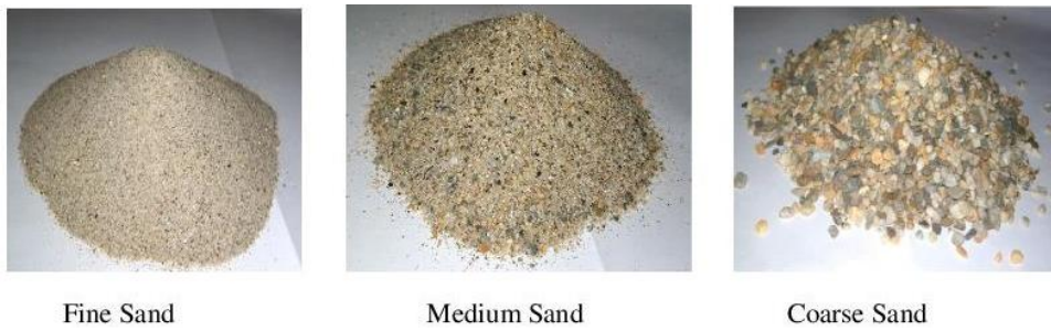
Figure 1. Fine, medium and coarse sands used in the direct shear test.
