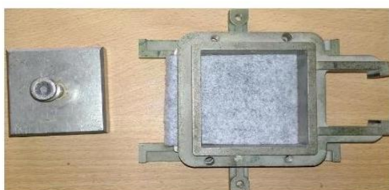
Modified shear box of which lower half is clamped with geotextile.
