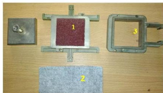
(1) Wooden block placed in lower half of shear box; (2) Geotextile; (3) Upper half of shear box.
