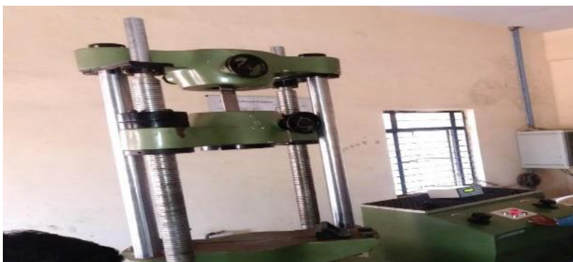
Figure 7. Universal testing machine.
