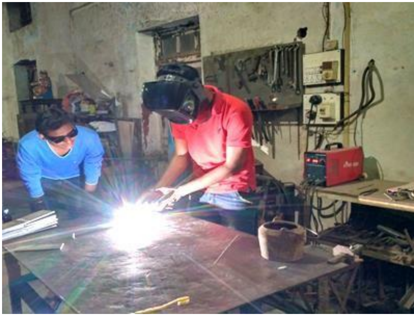
Figure 5. Welding of two pieces of SS304L.
