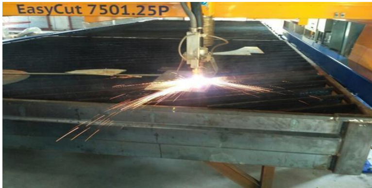
Figure 3. Metal cutting by using plasma arc machine (PAM).
