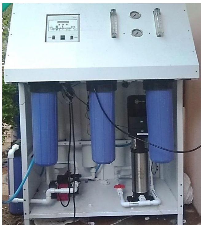
Figure 5. Highly compact cascaded membrane based DM Medical grade water production unit (500 L/h capacity).
