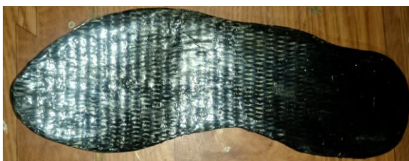
Figure 3. Carbon fiber Partial Foot Orthosis.
