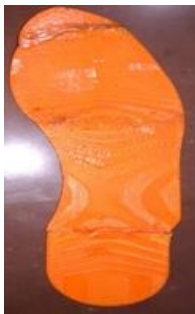
Figure 1. 3-D printed template to manufacture carbon fiber foot plate.
