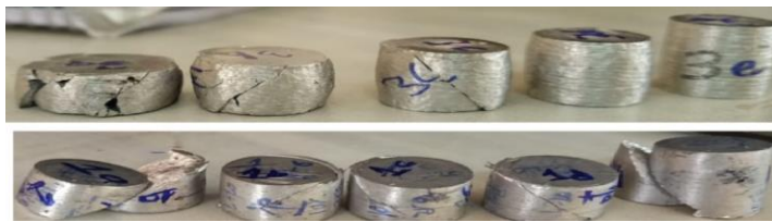
Figure 4. H/D 1.0 and 1.5 compression sample sets.
