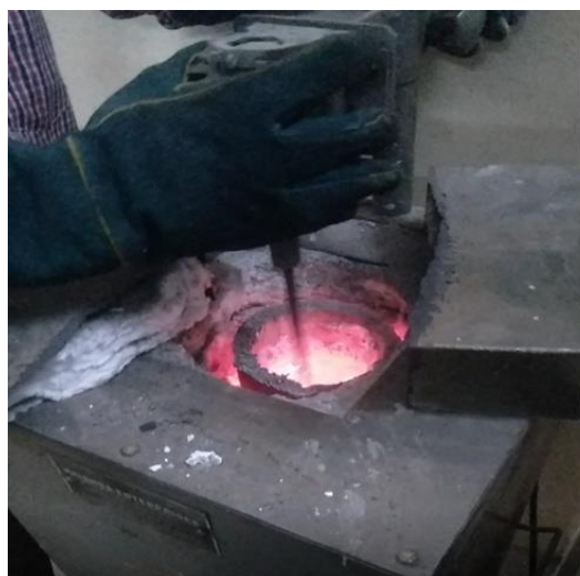
Figure 1. Samples of Stir Casting for Casting.
