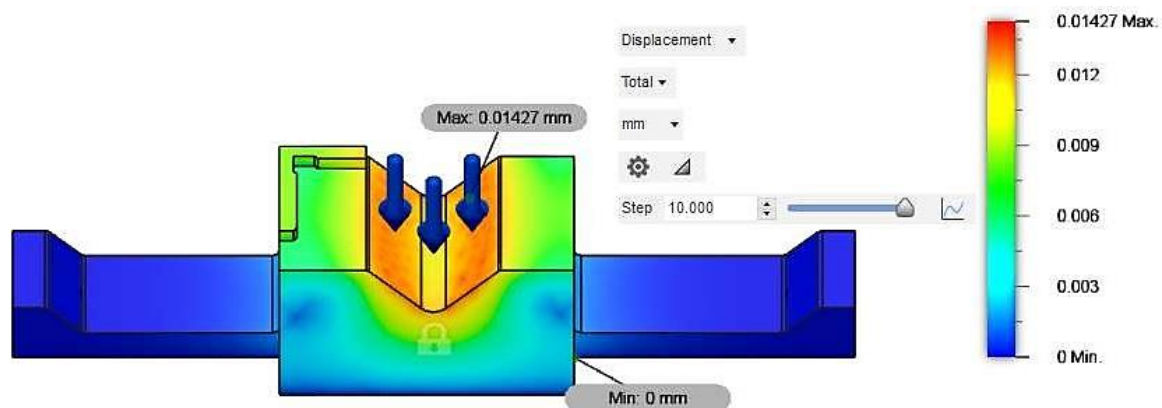
Figure 14. Deformation of Die
