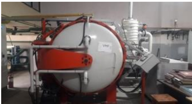
Figure 1. Vacuum Hardening (VH).
