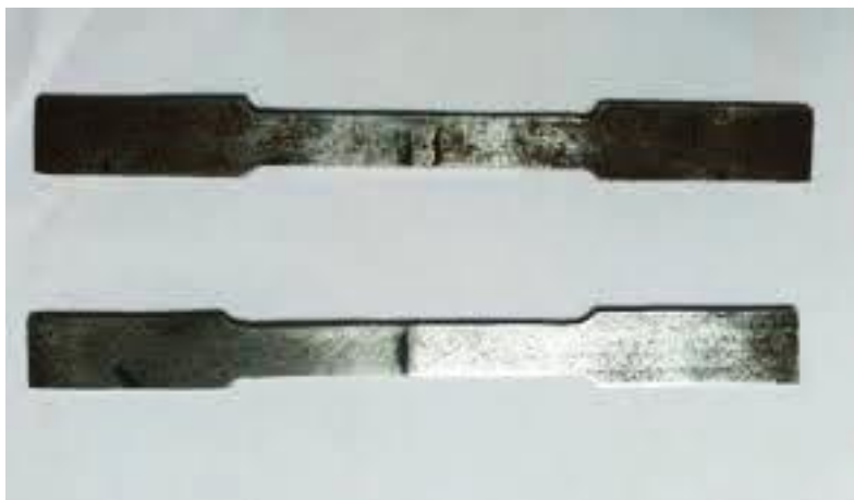
Figure 5. Weld samples by SAW (Submerged Arc Welding).
