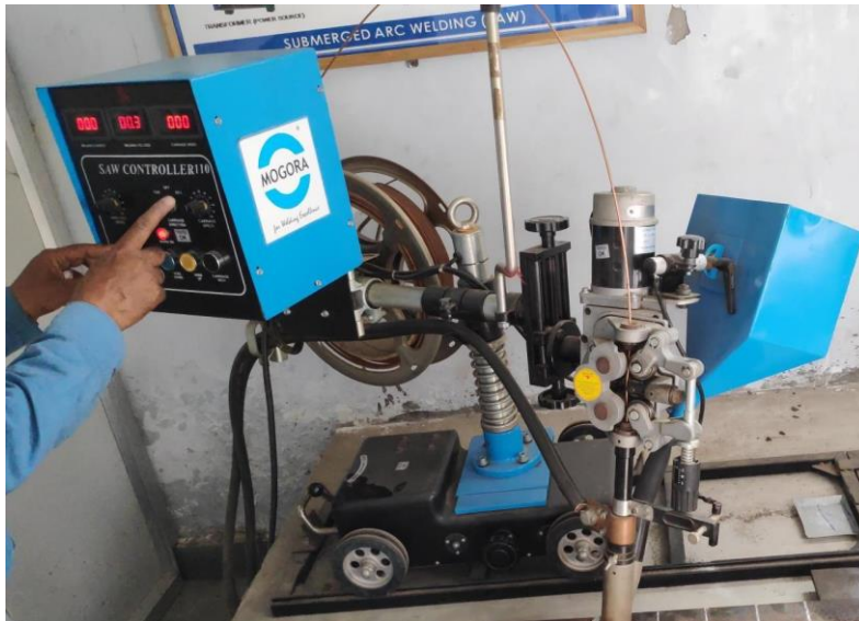
Figure 4. Submerged Arc Welding for Experimental Study.
