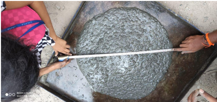
Figure 2. Measuring of Slump Flow for SCCC (source: pic taken at PVPSIT).
