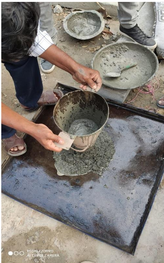
Figure 1 Slump Flow Test for SCC (source: pic taken at PVPSIT)
