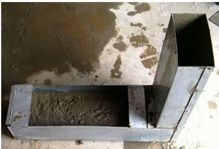
Figure 4. L-Box Test for Self-Compacting Composite Concrete (source: pic taken at PVPSIT).
