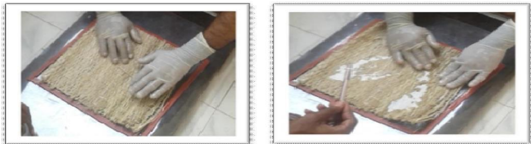
Figure 4. (b) Spreading of fibers on resin and resin on fibers.
