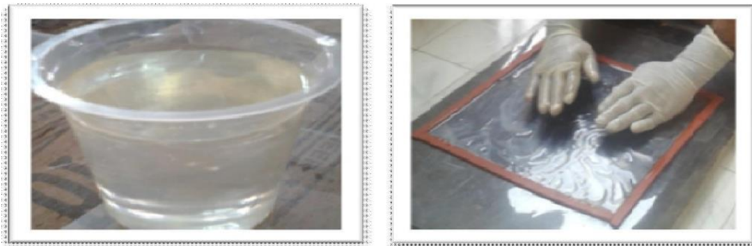
Figure 4. (a) Mixing of Resin and hardener with lamination sheet
