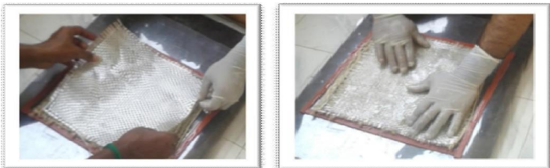
Figure 4. (c) Fixing glass fibers on resin and resin on glass fibers.
