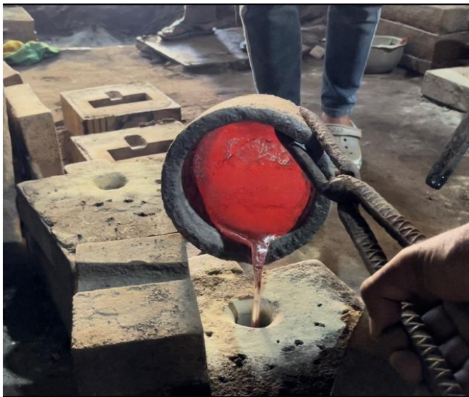
Figure 3. Pouring molten metal to the sand mold.
