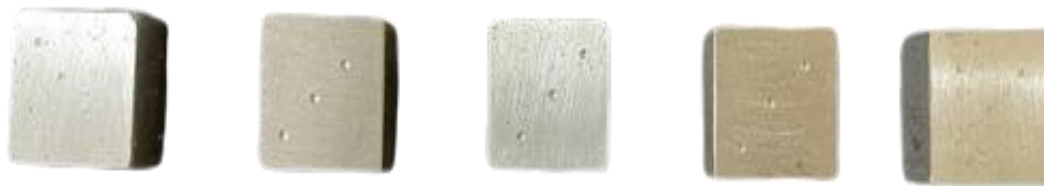
Figure 8. Specimen After Conducting Hardness Test.
