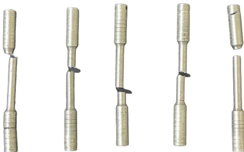
Figure 6. Shows broken specimens after tensile test.
