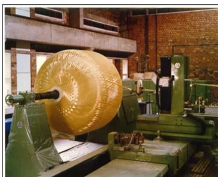
Composite Casing made through filament winding process
