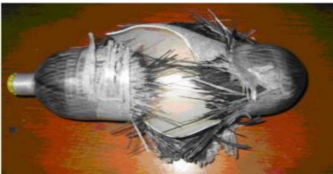
Figure 10. COPV after the burst test [28].
