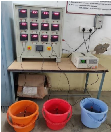
Figure 13. Corrosion resistance Apparatus (Samples with applied voltage).
