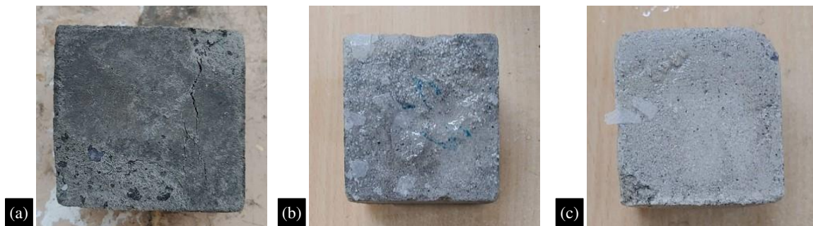
Figure 6. (a) Cement Block (Control) (b) Steel slag-Cement block (c) Steel slag Lime blocks.
