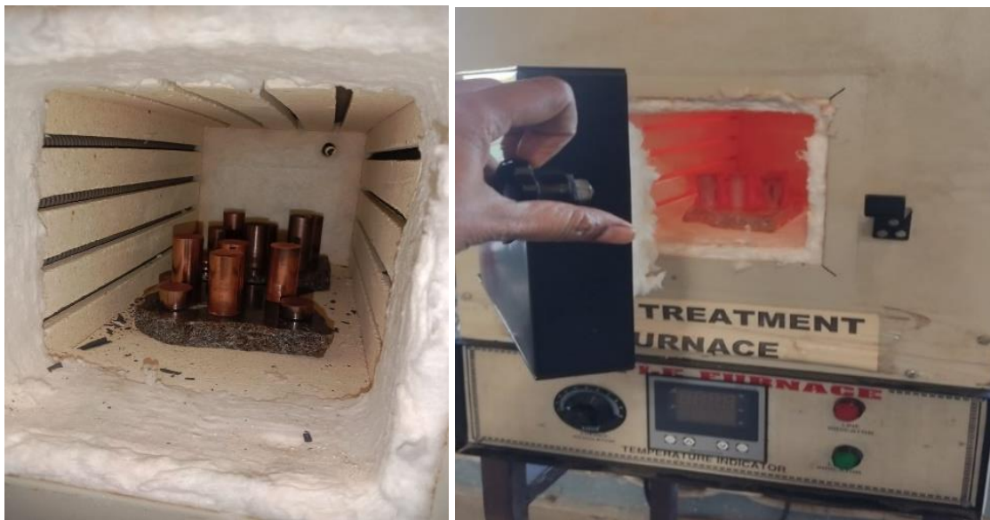
Figure 2. Green compact and furnace set-up.
