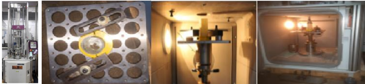
Figure 3. Impact Testing Machine, Test specimen on the base plate and with Tup.
