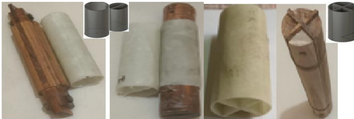
Figure 1. Multicell structure with mandrels.
