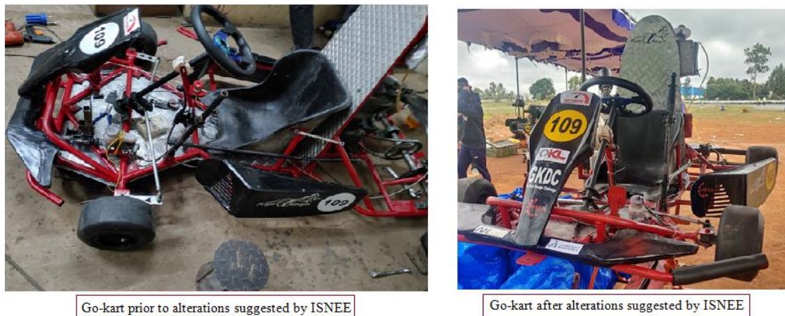
Figure 14. Go-kart prior to and after alterations suggested by ISNEE.
