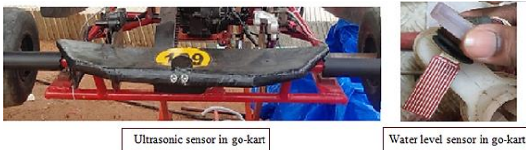
Figure 12. Ultrasonic and water level sensors in go-kart.
