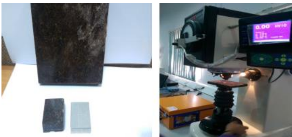
Figure 5. Hardness testing of date palm fiber laminates.
