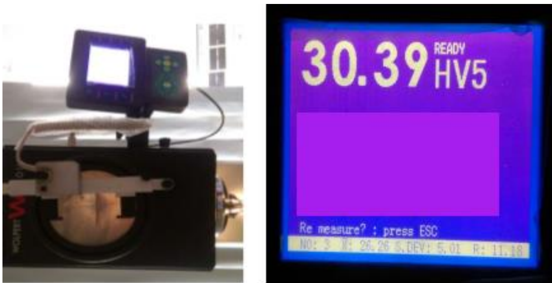
Figure 6. Hardness testing of date palm reinforced epoxy laminates.
