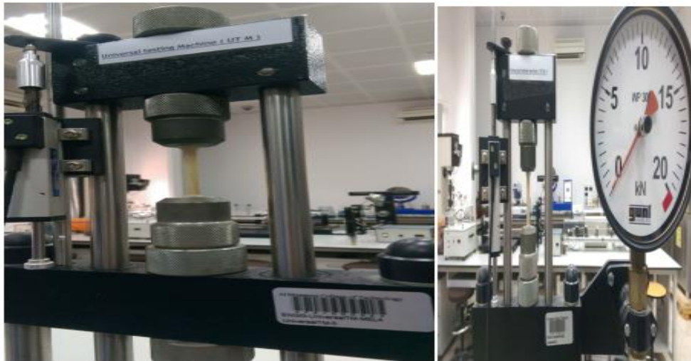
Figure 4. Preparation and testing of date palm fiber laminates.
