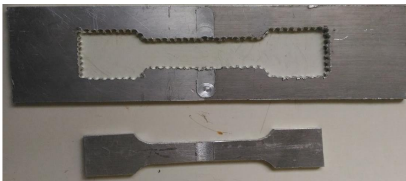
Figure 9. Specimen cut in I section as per standard [14].
