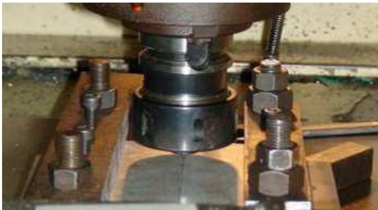
Figure 6. Centering the tool on the work piece joining line [15].
