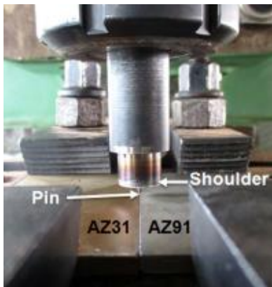
Figure 1. FSW process for butt welding [19].
