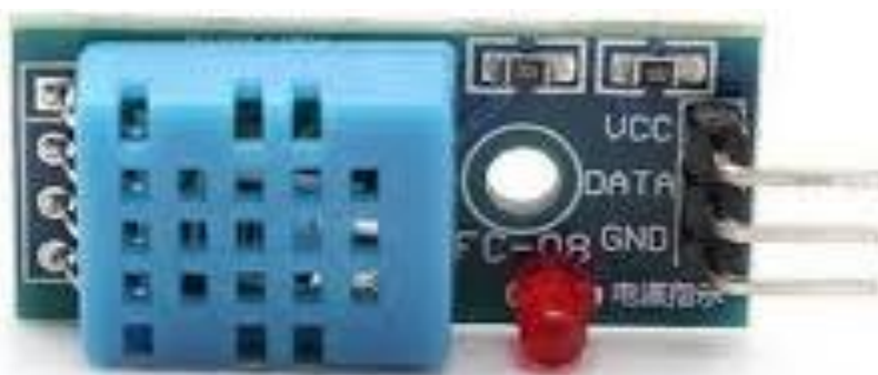
Figure 3. Temp and Humidity (DHT11) sensor [1].
