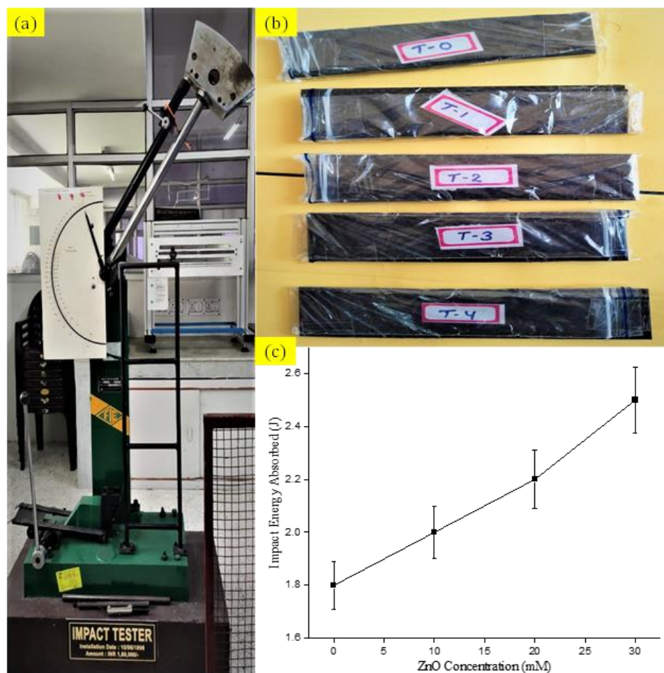
Figure 5. (a) Charpy impact test setup (b) Fabricated ZnO-WCF/Epoxy resin hybrid composites and (c) Impact energy absorption of laminated composite samples.
