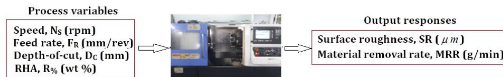
Figure 3. Process variables and output responses in the machining process.
